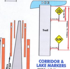
**ORANGE** (Tremdad Real Orange or Equivalent) 35mm in dia.(1.25") minimum 1.25m to 2m in height 35mm sq WHITE REFLECTOR(1sq. ") (min.) PLACE APPOX. 6cm (2") DOWN FROM THE TOP ON TWO SIDES FACING TRAIL, (Min.) USE MINIMUM - SINGLE ROW - TO DIVIDE A LAKE TRAIL, USE MINIMUM DOUBLE ROW TO MARK A FIELD TRAIL. INSTALL TRAIL ENDS SIGN WHEN TRAIL TERMINATES AT NON-STAKED LAKE. Conform by Oct. 15, 2004.
